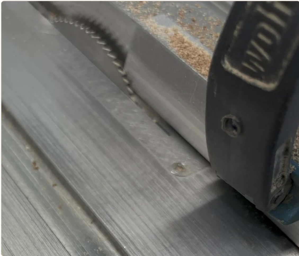
Close-up: L-angle sitting just above the table surface, teflon tape visible on the contact face.
