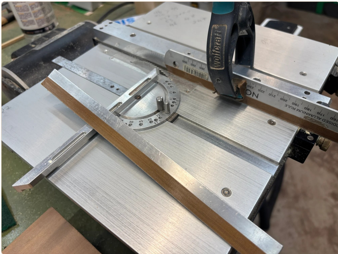
Full setup overview: L-angle and ruler clamped to fence, hold-down clamp in position.
